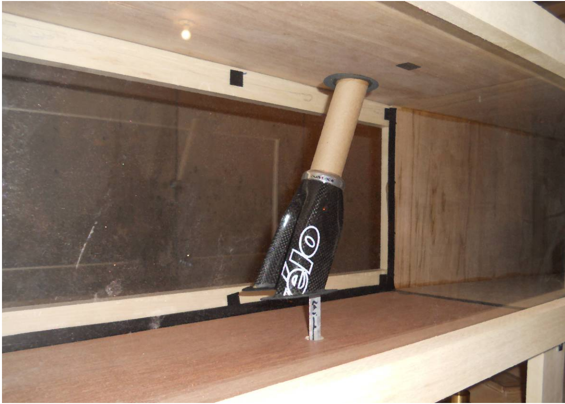
Figure 2. Brake sting constructed out of truncated Cervelo Wolf fork.
